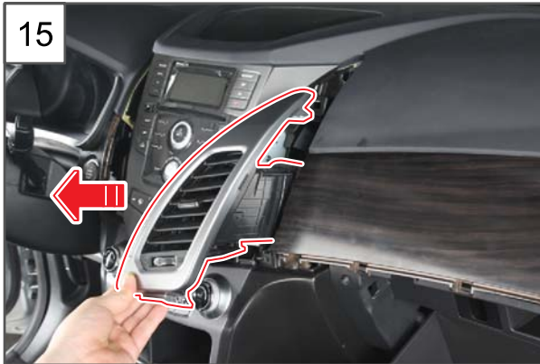
15.Remove the RH center fascia panel.
