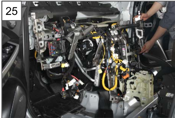
26. Unscrew the air conditioner module mounting bolt and mounting screw fitted to the instrument panel frame and disconnect the wiring connector.
