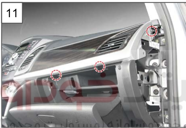
11. Open the glove box and unscrew the 3 mounting screws securing the RH side fascia molding.
