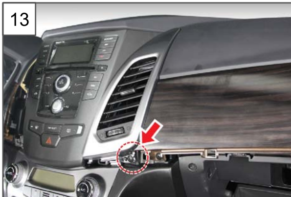
13. Unscrew the RH center fascia panel mounting screw.
