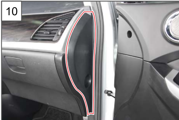
10. Remove the RH crash pad side cover.
