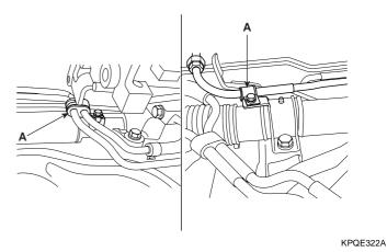
11. Remove the mounting clamp of power steering gear box, and also remove the clamp holding the pressure tube and the return tube.
