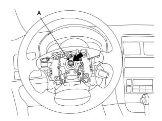
Remove the steering wheel lock nut(A).
