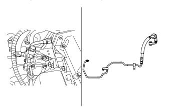
Fix the return hose(A) and pressure tube(B) fitting to the power steering gear box.
