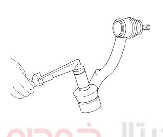
4. If the starting torque exceeds the upper limit of the standard value, replace the tie rod end.
