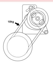
Put a bar(A) or equivalent, between the bracket(B) and the oil pump(C) and adjust the tension so that the belt deflection is within the standard value.
