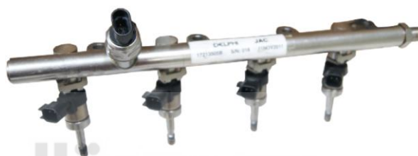
Figure 4-31 Fuel injector installation position
