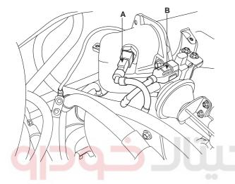
4) Three fuel injector connectors(A).
