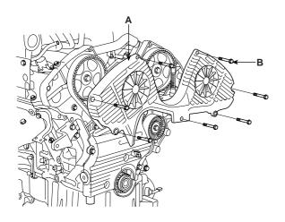
17. Install the engine mount bracket.
