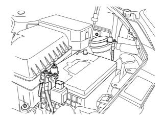
Disconnect the negative terminal from the battery.
