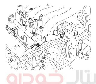
18. Install the brake booster vacuum hose(A).
