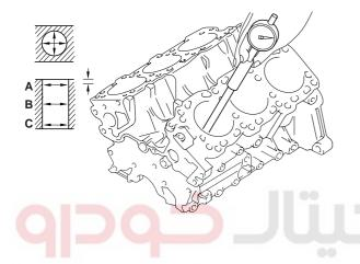
Check the cylinder bore size code(A) on the cylinder
