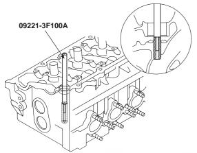
Using the SST(09221-3F100A/B), press-fit the valve guide. The valve guide must be press-fitted from the upper side of the cylinder head. Keep in mind that the intake and exhaust valve guides are different in length.
