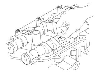
If the oil clearance is greater than maximum, replace the camshaft. If necessary, replace the bearing caps and cylinder head as a set.
