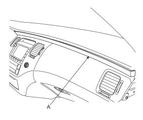
Loowen the screw. Remove the center facia pannel (A) and then disconnect the connectors.
