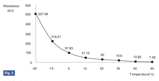
Fig 3) Specifications: Resistance value of ambient temp. sensor as a function of temperature.
