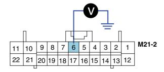
6. Evaporator temp. sensor signal
