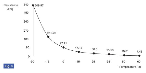
Fig 3) Specifications: Resistance value of incar temp. sensor as a function of temperature.
