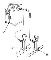
If the low-pressure does not reach more than 93.3 kPa (700 mmHg, 27.6 in.Hg) in 10 minutes, there is probably a leak in the system. Partially charge the system, and check for leaks (see Leak Test.).
