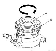
4. Check operation of the magnetic clutch.
