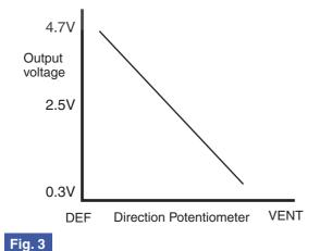
Fig 3) Specifications: Voltage value as a function of position of direction potentiometer.
