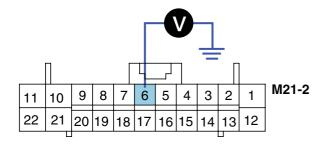
6. Evaporator temp. sensor signal
