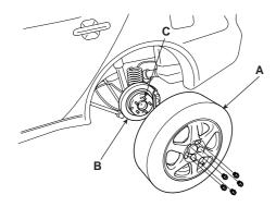
Remove the rear shock absorber assembly nut(B) from the rear knuckle, then remove the shock absorber assembly(A).
