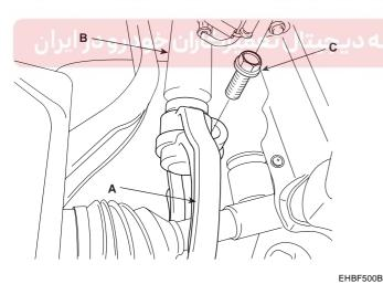
Install the fork(B) to the front lower arm(A) connecting bolt(C).
