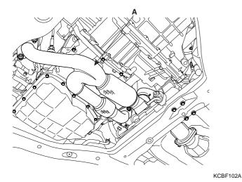
29. Supporting the cross member(A) with a jack, remove the stay with the mounting bolts.
