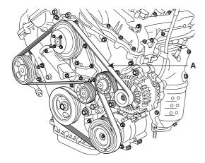
2. Remove the power steering pump(A).
