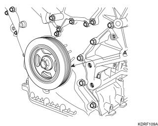
Remove the timing chain cover(A).
