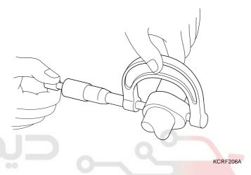
If the cam lobe height is less than standard, replace the camshaft.
