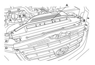
6. Remove the radiator bracket(A).
