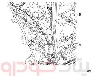
16. Install oil pump chain guide(A).
