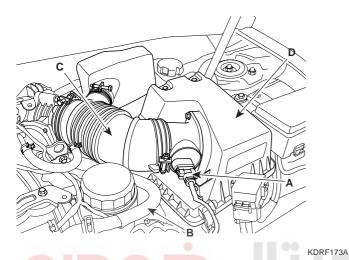
3. Disconnect RH oxygen sensor connector(A).
