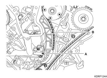
21. Remove tensioner adapter assembly(A).
