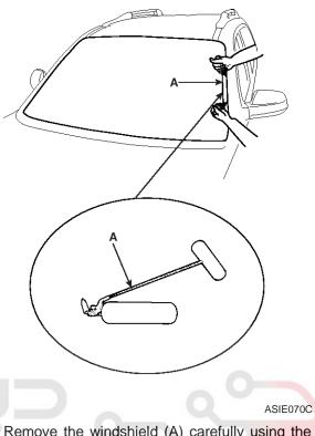
4. Remove the windshield (A) carefully using the glass holder (B).
