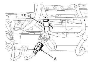
5. After removing the tape (B) on the front of seat back remove the seat cushion cover (A).
