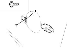
3. After loosening the door module mounting bolts and screws, then remove the door module (A).
