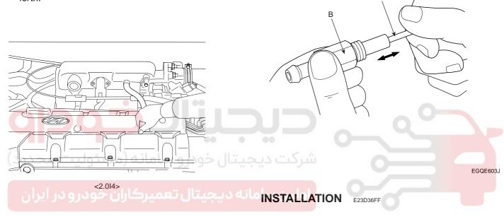
Install the PCV valve and tighten to the specified torque.
