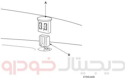
Disconnect the 8P connector (B) from the auto light unit then inspect the connector on the wire harness side, as shown in the chart.
