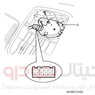
3. Ground the terminals as below table, and check that the sunroof unit operates as below table.
