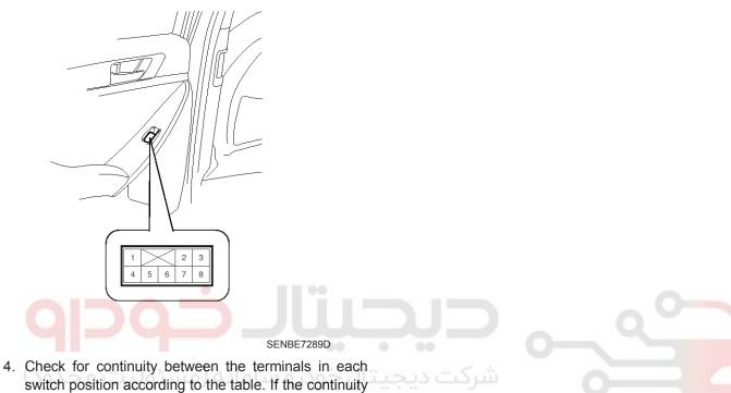
condition is not normal, replace the switch.
