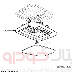
1. Install the room lamp assembly after connecting the
