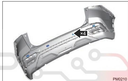
5. Remove reversing radar sensor from slots of rear bumper assembly.
