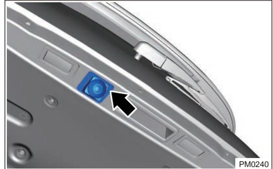
5. Disconnect rear camera connector, pry up fixing clip (1) from camera connector and remove rear camera.
