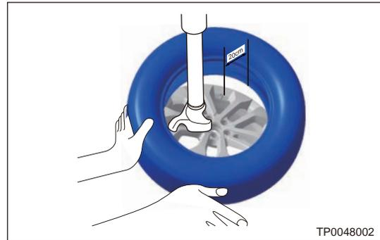
7. Rotate wheel to install another side of tire into hub.
