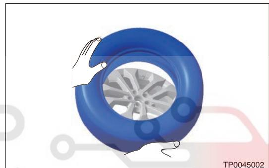
4. Install bottom tire to make sure the distance between intersection and valve stem is about 20 cm.
