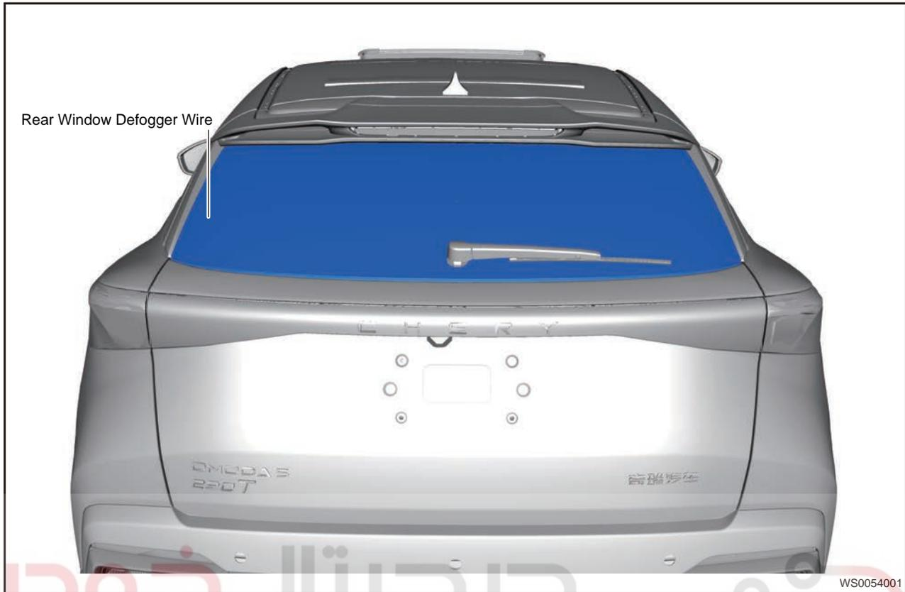
Turn on the rear defroster switch, heat the rear defroster heat wire to remove fog, frost or water steam on the rear windshield, gaining clear view. To turn on the rear defroster, it is necessary to turn ENGINE START STOP switch to “ON” and press rear defroster switch. Rear defroster switch indicator comes on, while the indicator on rear defroster switch starts to work. Rear defroster stops operating and the indicator goes off after the rear defroster switch is pressed again.
