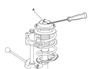
3. Using the special tool (09546-26000), compress the coil spring(A) until there is only a little tension of the spring on the strut.
