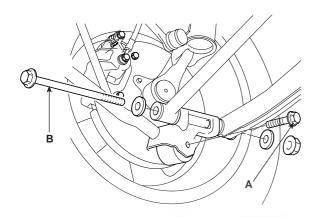
Remove the suspension arm bracket mounting bolts(A).
