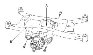
9. Remove the suspension arm(B).
