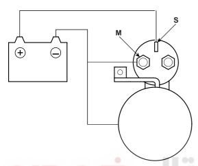
Disconnect the battery also from the body. If the pinion retracts immediately, it is working properly. To avoid damaging the starter, do not leave the battery connected for more than 10 seconds.
