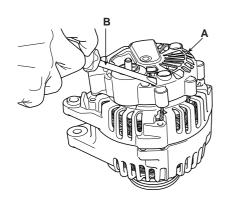
5. Remove the nut, pulley(A) and spacer.
