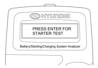
Cranking voltage and starter test results will be displayed on the screen.
