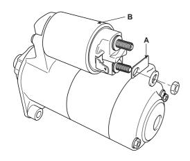
Remove the brush holder assembly (A), yoke (b) and armature (C).
